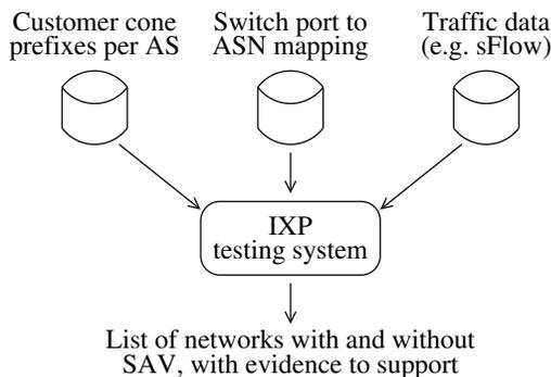
Figure 3: *Architecture of IXP-based testing system. Using CAIDA’s customer cone inferences, a mapping of switch ports to ASes, and traffic data, we can infer which networks have deployed SAV.*
