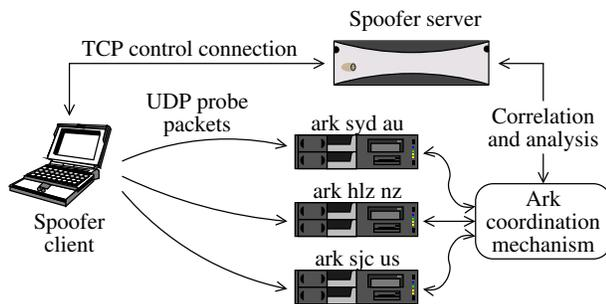
Figure 1: Architecture of current client-server testing system. Spoofed and unspoofed UDP packets are sent to a distributed set of Ark nodes to test the ability to send spoofed packets, as well as where along a traversed path SAV might be taking place.
