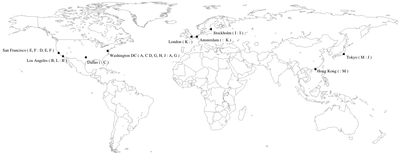
Fig. 1. Location of root and gTLD servers. Each city lists servers (root : gTLD) using their one-letter names. Note the uneven geographical server distribution, with high concentrations on the US East and West Coasts.
