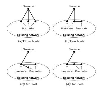
FIG. 3: Link placement options for three links.
