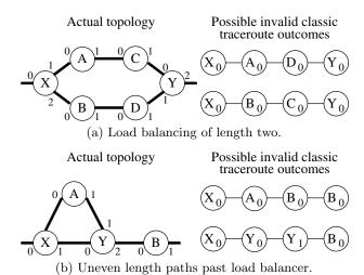
Figure 1: Load balancing can cause false inference of router-level links. In 1(a) links  $A_0 \to D_0$  and  $B_0 \to C_0$  are invalid as the routers are not adjacent. In 1(b)  $A_0 \to B_0$  is invalid as the routers are not adjacent, and  $Y_0 \to Y_1$  is invalid as the addresses are aliases.
