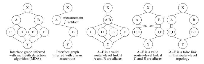
Figure 2: Classification of measurement artifacts in an interface graph. A measurement artifact introduces error into the router-level topology if it connects two routers that are not neighbours.
