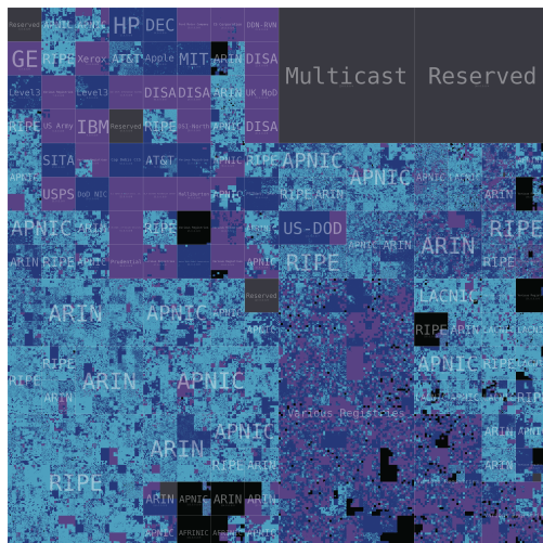
Fig. 8: Hilbert map visualization showing the utilization of the address space according to our taxonomy. The IPv4 address space is rendered in two dimensions using a space-filling continuous fractal Hilbert curve of order 12 [53], [58]. Each pixel in the full-resolution image [17] represents a /24 block; light blue indicates used, dark blue routed unused, purple unrouted assigned, black unassigned, and grey reserved by RFC blocks.
